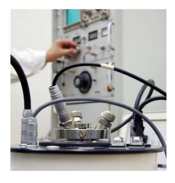
Testing POWERSIL® Fluid TR20. The newly developed insulating fluid has a very low viscosity and excellent cold start capabilities. This guarantees reliability when used in electrical machinery, including power generators. (Photo: Wacker Chemie AG)
