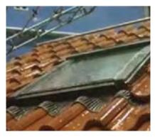
Severe wind and rain test in the VELUX wind tunnel.
