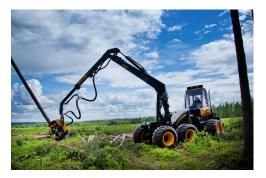
Eight wheels and articulated frame steering create a flexible and stable machine with high capacity, low ground pressure and excellent operator comfort. With tracks at the back and front plus new cranes, the result isn't a long way from the ultimate machine of every contractor's dreams.
