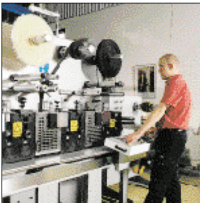
Rotary stamping of display covers.
