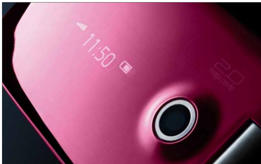
Mobile phones are given a shiny surface using vacuum metallization.
