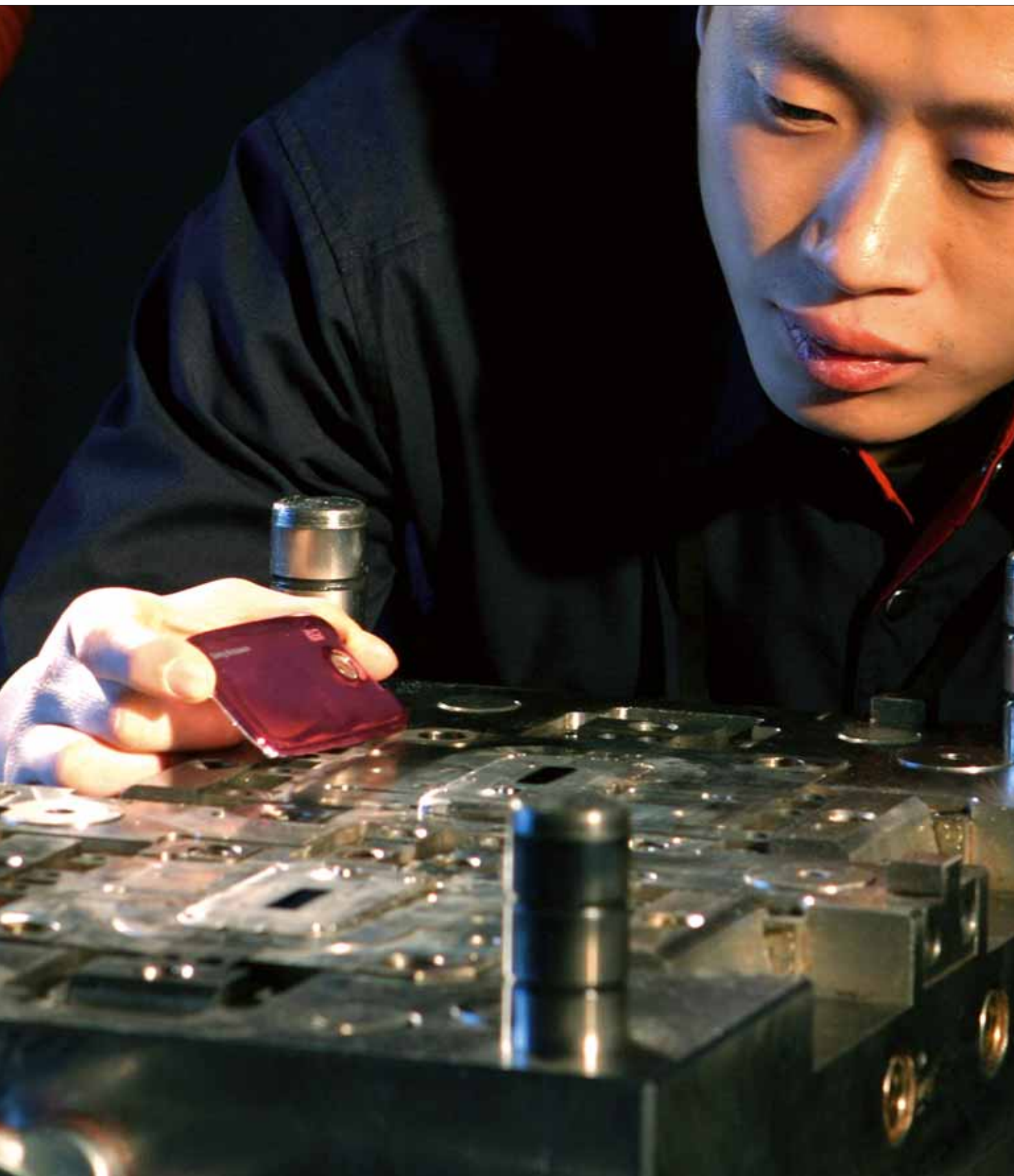
Having its own mould manufacturing is a strategically important part of Nolato Telecom's customer offering. JiHong Cao, Nolato Beijing, checks a mould for a mobile phone front.
