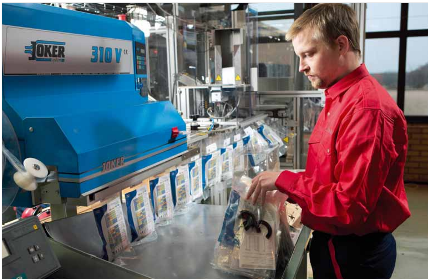
Joakim Svensson, Nolato Polymer, Torekov, Sweden, monitors the fully automated process for manufacturing bearing housing seals for SKF.
