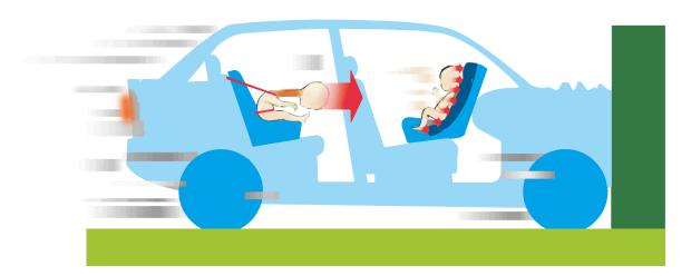
Figure 2. The load to the head and neck in a rear-facing and forward-facing CRS
