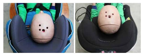
Figure 6. Left: Deep side wings. Right: Shallow side wings
