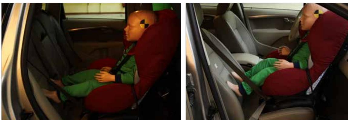
Figure 3. A CRS mounted in frontal and rear seat of a Volvo V70
