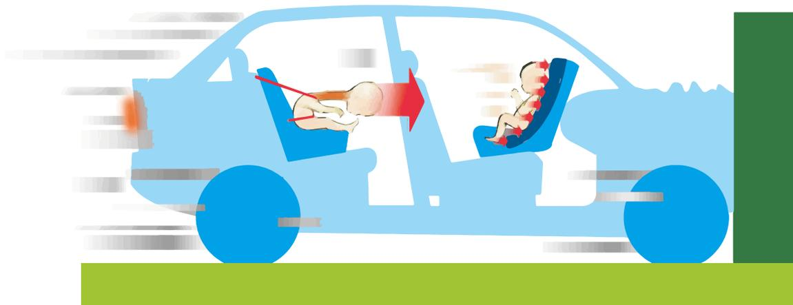
**Figure 2.** The load to the head and neck in a rear-facing and forward-facing CRS
