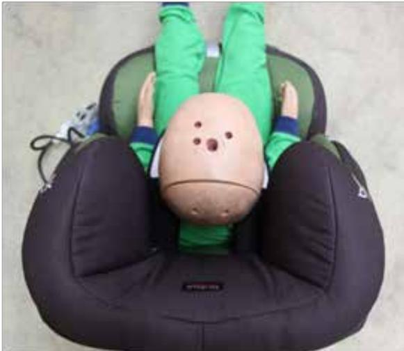
Figure 7. An example of a good side protection, Britax Römer Multi Tech II
