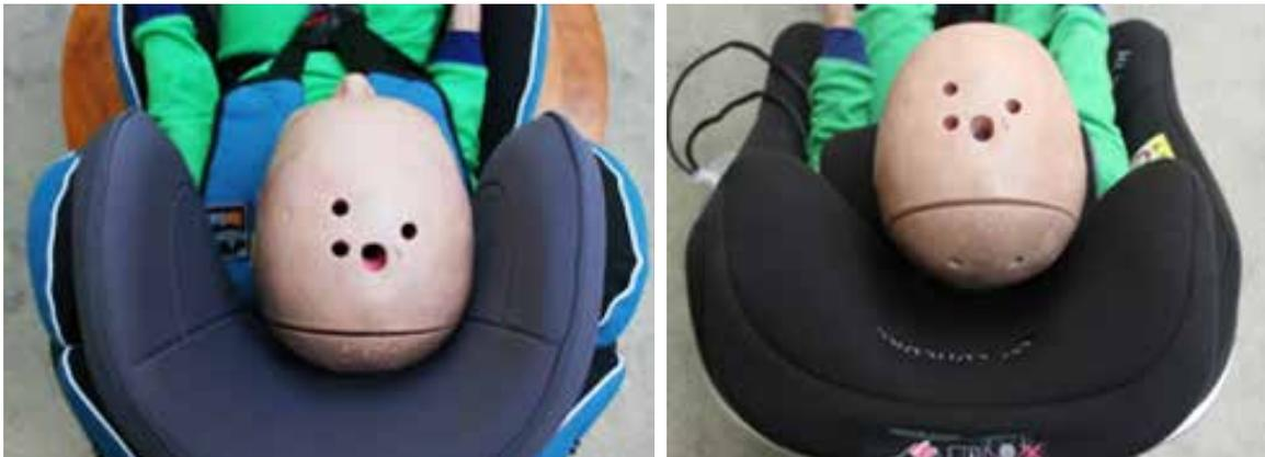
Figure 6. Left: Deep side wings. Right: Shallow side wings
