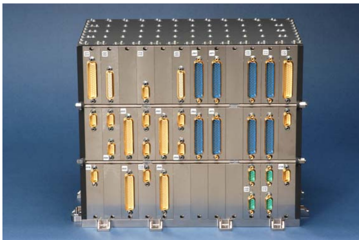
Herschel/Planck Attitude and Orbit Control Computer, ACC.
