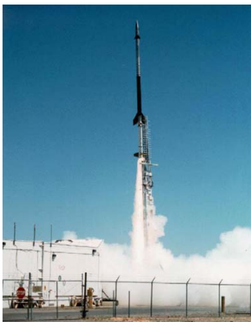
A NASA research rocket is launched. The guidance system control fins are seen near the top of the rocket.
