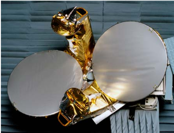
The Gregorian earth deck antennas dressed in thermally protective foils
