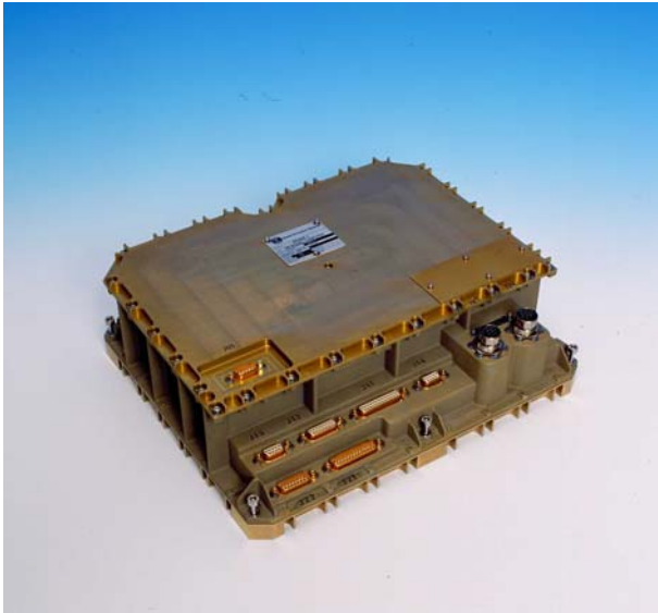
Two computers like this are working in parallel during each Ariane-5 launch.
