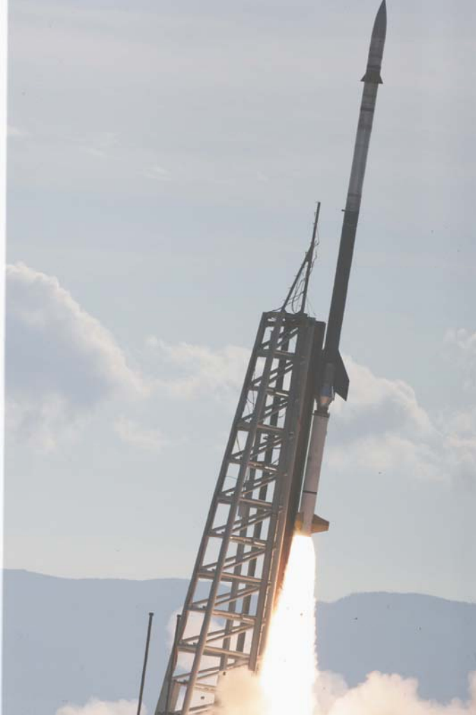
The Terrier-BlackBrant sounding rocket takes off on its first mission guided by the upgraded S19L system.
