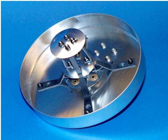
SMART-1 Patch Excited Cup Antenna, similar to the ones now on order for LCROSS.
