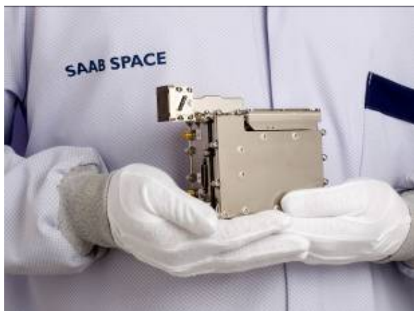
Ku-band receivers of the type now ordered by Orbital Sciences.
