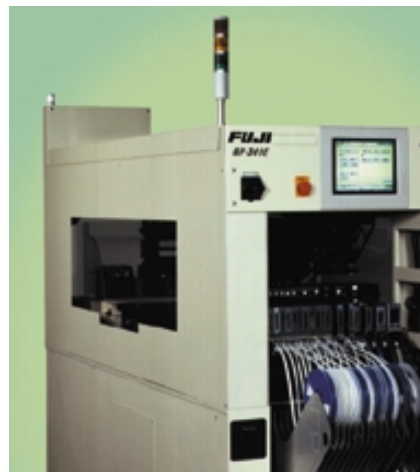
Fuji OP3 – one of the most versatile machines on the market for surface-mounting components and connectors.
