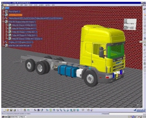
Digital Mock-Up, Scania R144, three months before production
