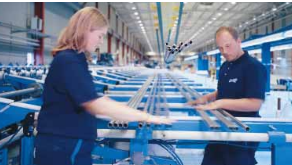
The new assembly line for heat-exchanger tubes that was installed in Sandviken during the year will mean considerably shorter production time.
