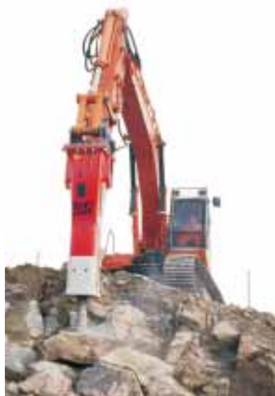
Rammer's hydraulic hammer is used for rock crushing and demolition.
