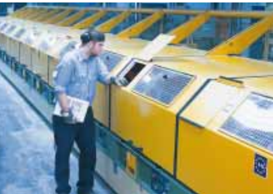
A new dry drawing machine improved productivity at the Kanthal plant in Hallstahammar.
