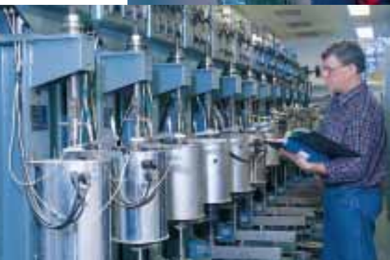
1. Furnace for diamond coating of cemented-carbide inserts at Sandvik Coromant in Västberga, Stockholm.
