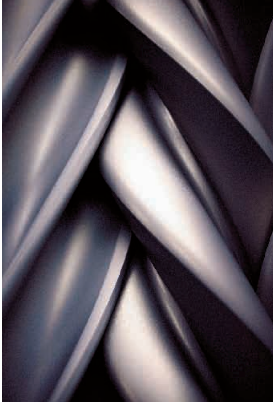
A pair of rotors for a screw compressor in close-up. The rotors rotate at around 15,000 revs per minute with an air column between them. The air is moved and compressed at the same time, boosting the compressors efficiency.
