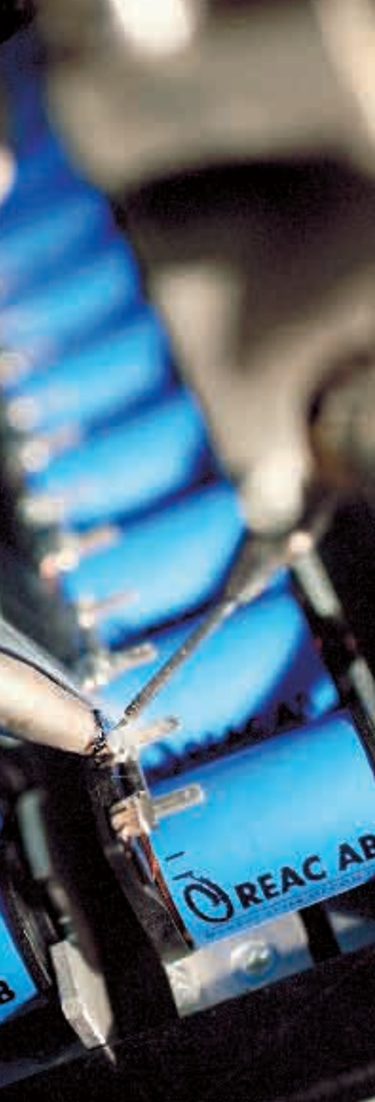
Left: Items previously soldered by hand are now soldered by robot in a fully automated process.
