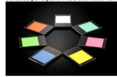
A VELVE OLED evaluation kit is also available. It consists of a colour-tunable, framed OLED measuring 207 x 145 x 18.3mm and an electronic circuit controlled via an USB connection. The initial colour and white tones are pre-programmed.
