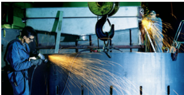
▲ Grinding of stainless steel cylinder holders.
