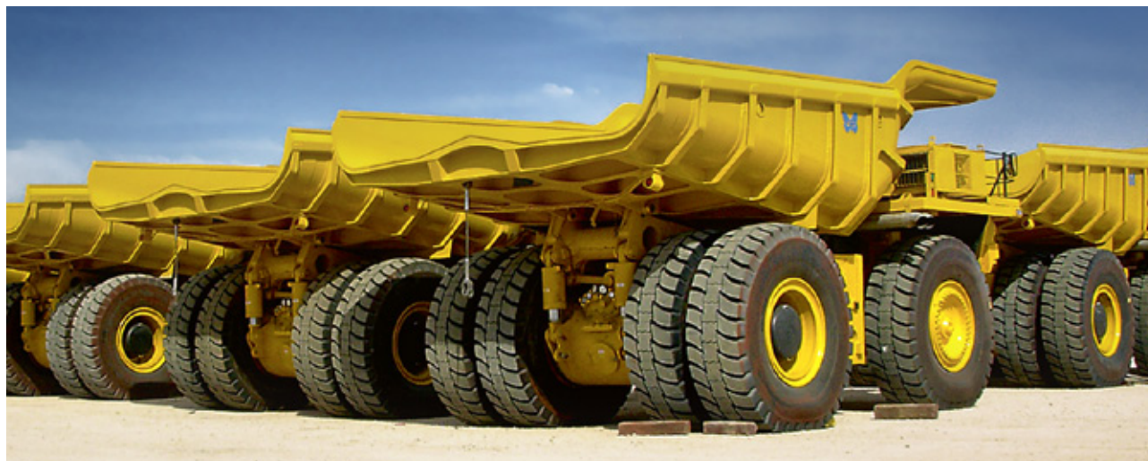
▲ Dumper trucks with a bed made of high strength steel from SSAB.
